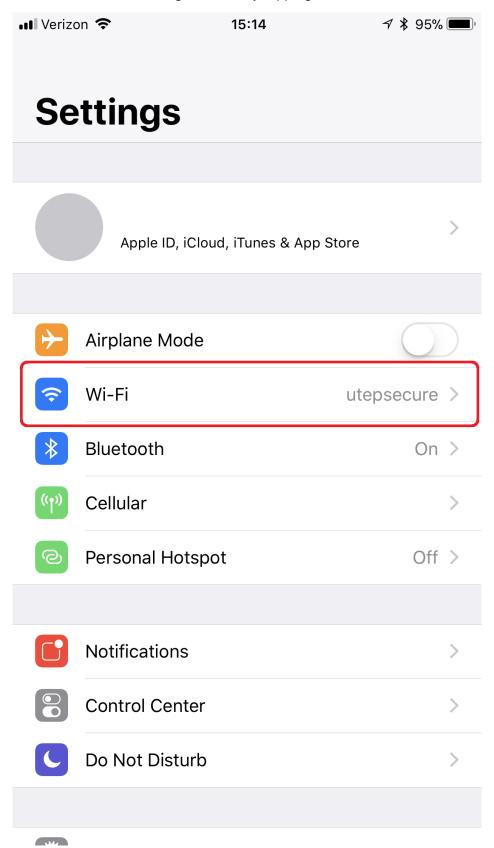
3. Under the wireless settings, choose the network that you want to forget. For UTEP's wireless network, the network name should be *utepsecure*. Tap on the '*i*' button next to the network name to select it.
