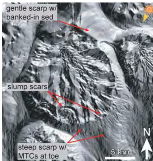
Fig. 9. Dip-azimuth image of seafloor over Mica salt body in Mississippi Canyon, northern Gulf of Mexico (MTC: mass-transport complex). Illumination is from upper right such that NE-facing slopes are lighter and SW-facing slopes are darker. Seismic data owned by TGS, image courtesy of E. Mozer and Samson Offshore.
